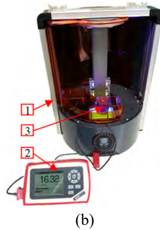
Figure 2-4(a) A projected image with nine 10 \times 10 mm squares having 155 grayscale pixel value, (b) measuring the irradiance of the Ember machine using a power meter
